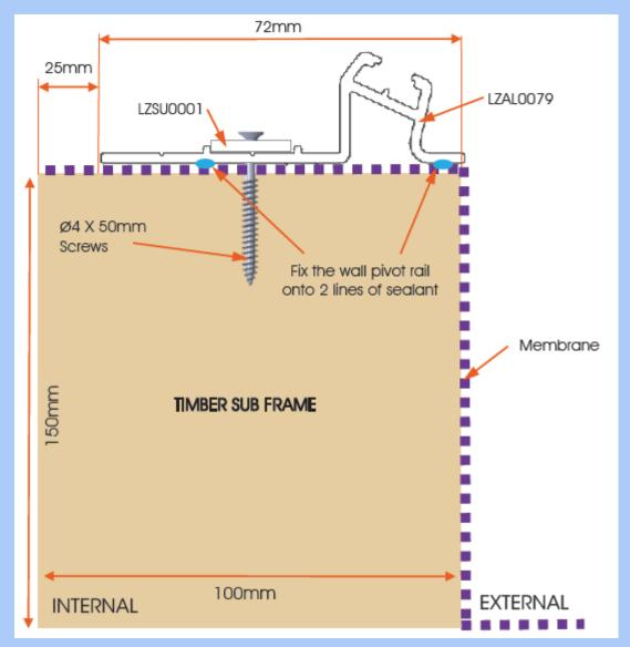
Drill holes in Wall Rail for 90° Horizontal Joining Plate. Use this as a template for hole position. Apply silicone to sub frame and fix Wall Rail with Ø4 x 50mm screws.
