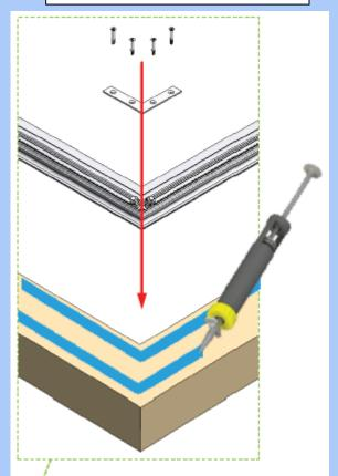
Drill holes in Wall Rail for In-Line Horizontal Joining Plate. Use this as a template for hole position. At the same time as the 90° Horizontal Joining Plates, apply silicone and fix Wall Rail with Ø4 x 50mm screws.
